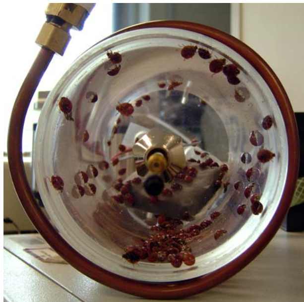
Fig. 1 Environmental sampling chamber. This is a 1-l plexiglas cylindrical container, encircled with copper tubing connected to a water bath to control temperature. A small, mesh-covered, battery-operated fan is housed inside the chamber to maintain homogeneous air circulation. The chamber is equipped to accept SPME fibers and an air tube for whole air sampling
