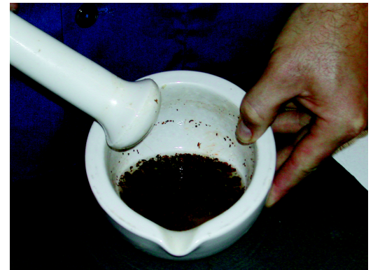
Fig. 3. One hundred MALB crushed in 100 mL of wine. After centrifuging and filtering, this mixture was used to "spike" the test wines for sensory detection limits with consumer panels. (Photo: J. Kovach)
