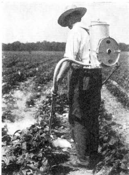
FIG. 8.—BELLOWS TYPE OF HAND DUSTER SUITABLE FOR DUSTING SMALL PLANTINGS. (Photo by N. F. Howard, United States Department of Agriculture, Bureau of Entomology.)
