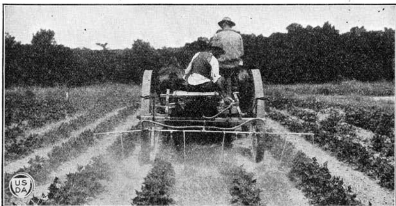
FIG. 12.—Spraying beans for the Mexican bean beetle with a power sprayer. This machine may be adapted to spray 8 rows at once.
